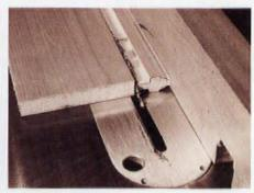
ABOVE: A combination plane cuts the muntin detail. RIGHT: I had to grind the blade to the profile I needed. FAR RIGHT: It's easier to work from the edge of the board and cut it off last.
