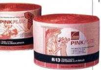
Plastic-wrapped fiberglass insulation is available in R-13 with kraft facing for walls, and in R-25 for crawl spaces and attics.
