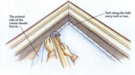
Once it has been secured along the bottom of the gable, lift the canvas to the gable peak and tack the top point into place. While an assistant pushes with a board, fold the edges over and secure the canvas to the sheathing.
