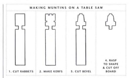
passes on the table saw and adjusting the blade height so the kerfs take on the basic profile of the moulding you are attempting to reproduce. Hand rasp and sand the rough shaping into the proper detail.
