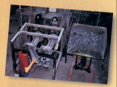
■ V STEP 3: The heart of the machine is the moving head knife (photo below). This carbon-steel tool, sharpened like a wide chisel, cuts a nail each time it travels
