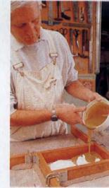
Pour the rubber in a small, steady stream so it flows smoothly over the model without trapping air in the crevices.
