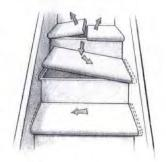
Then fabricate a new tread. cutting it just the distance between the stringers, plus the 1/2" into the mortise probably 1/4" shorter than the original tread. If you've measured closely and cut accurately, you should be able to "shoehorn" one end of the new tread into the deepened stringer, then pull it over into the other stringer mortise. Last, toenail the tread into the stringers with finishing nails.
