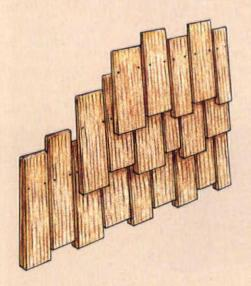
Sawn, perfection shingles, selected for regular widths and staggered a standard, single dimension will create a buttline as precise as a wave on an oscilloscope. Random-width shingles staggered at more than one dimension will look free-form.
