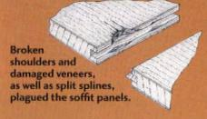
It was simple enough to replace the split and missing splines with new, solid oak stock, but the dadoes had to be repaired too. We used a two-part epoxy wood filler system to rebuild these grooves. The filler is applied in a thick, puttylike state and can be tooled with common woodworking equipment. (Epoxy consolidant will reamalgamate crushed wood.) Compared with a wood dutchmen the
