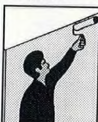
12. Apply 2nd coat of saturant (include seam).
