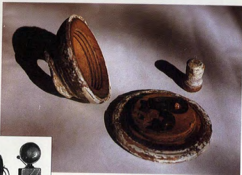
Above: A wood push-button doorbell, from a 1920s bungalow. Left: This outfit retailed for $1.50 in 1907. The same setup with a metal push button cost $2.
