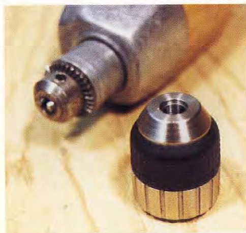
Although keyless chucks are larger and don't reach some of the tight places a geared chuck can go, they are easier to use.
