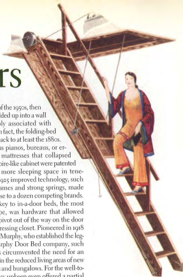
Sliding or folding stairs that stored in the ceiling came of age in the Roaring Twenties, and were among the most mechanical of built-ins (above). Rolling, tilting, sliding, and folding out of sight, mechanical space-savers like disappearing beds brought early-20th-century ingenuity to the built-in era (opposite).
