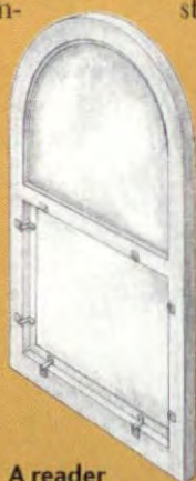
A reader retrofitted his exterior storms with a removable lower pane.
