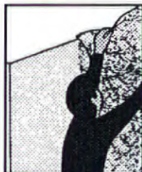
9. Apply mat to 2nd area, overlapping by 1".
