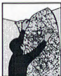
3. Apply fiberglass mat to wet surface.
