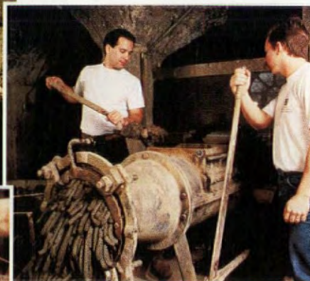
Mercer got his clay locally, primarily from the farmlands of Bucks County, which yielded a reddish-hued tile. The Tile Works still obtains local clay, supplemented by commercial products. The original pug mill processes the clay.
