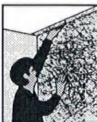
4. Trim excess mat where wall meets ceiling.
