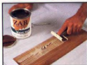
A graining tool and ZAR Stain create a rich wood-like finish on steel doors.
