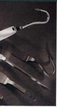
Use the curved hook to clear away any remaining stubs from the open deck. The slate ripper comes in 12" to 25" lengths and retails for \$68 to \$98. Shorter lengths are suited for smaller roofing slates and valley work; longer rippers work best with larger slates. Order from North American Böcker, 315 Capital Blvd., Raleigh, NC 27603, (888) 262-5371, or through dealers.
