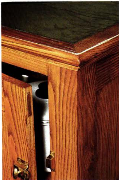
Above: Our new peninsula cabinet features mortise-and-tenon joinery. Right: Kerby checks the cut of a mortise for a stile.
