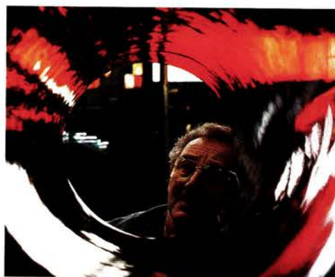
At Glashutte Lamberts in Germany, artisans still make mouth-blown cylinder glass. The process starts with a red-hot balloon of glass (1).
