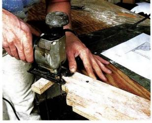
Left: Plowing the plywood-and-metal mould accurately through mounds of soft plaster takes a steady arm and a skilled eye. Above: For both the metal knife and plywood horse, a sabre saw cuts the pattern. Top right: Plaster is so fine that Henry must file away the smallest burrs in the knife or they'll show up in the moulding. Bottom right: The horse recessed from the knife; some moulds (top in photo) even have the wood relieved on the back for extra clearance.
