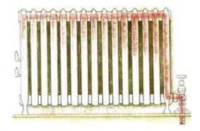
partially filled with a mixture of alcohol and water. He designed the alcohol/water mixture to boil at about 180 degrees F. Then he attached the float to a needle that could rise up and down and close the vent when the alcohol/water mixture "flashed" to vapor inside the sealed float. By 1921 Hoffman had sold more than 2 million Number Ones. Today's air vents are very similar in principle.
