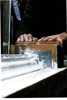
Below: In under an hour, a bucket of wet plaster has been transformed into 8' of moulding with skin-smooth curves and corners as sharp as glass. Bottom: A gentle nudge releases the finished moulding, and readies the bench for the next run.
