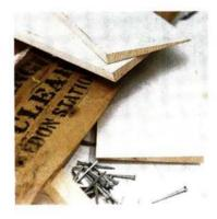
Meticulous Materials Like the 90-yearold spruce siding they replace, the new pine clapboards on this project are radially sawn, the traditional manufacturing method in New England. In this process, each board is cut from the log at right angles—like taking a thin serving of dessert from a pie. The result is a board with grain that is exactly perpendicular to the face of the board, giving the wood maximum weather and warp
