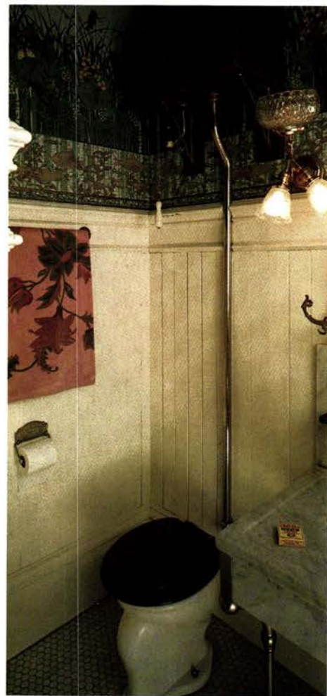
Above: Believe it or not, antique, pull-chain water closets can be adapted to meet low-flush building code requirements. Left: A single-leg pedestal sink saves space in a small bath.
