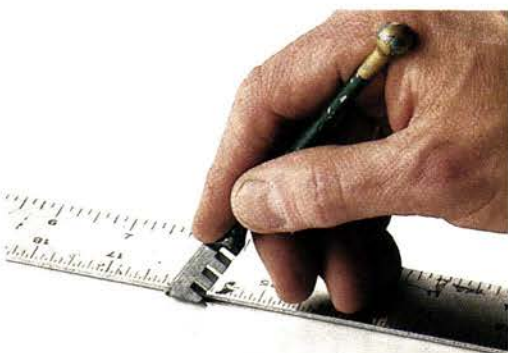
Top: First lubricate the wheel at the tip of a common glass cutter, then score the glass once in a thin white line. Below: Flex the end of the glass to snap the sheet in two.
