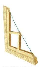
A true divided light is a window sash composed of individual panes of glass, held in a frame of wood muntins.
