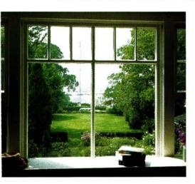
GLAZING The best way to reduce heat loss is by adding layers of glass. As more panes are added, the R-value increases. Two layers, or double-glazing, cuts heat loss almost in half. Triple-glazing cuts heat loss by two-thirds, but it also reduces light transmission by 10%.
