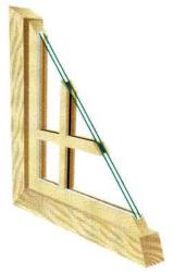
To simulate the appearance of true divided lights, manufacturers put a shadow or spacer bar between double glazing, then apply mock muntins on both sides of the glass.
