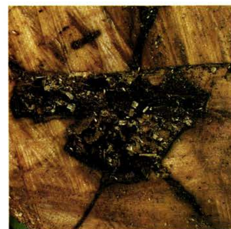
Top: Formosan termites literally shred wood in their search for life-sustaining cellulose. Originally from China, they have been in Hawaii for well over a century. The famed Iolani Palace in Honolulu, built in 1845, was so devastated by Formosans that it had to be taken down and totally rebuilt starting in 1879. Above: In New Orleans, Formosans infest live oak trees with no apparent visual signs.
