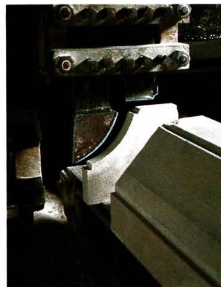
Left: A 76" diamond circular saw slices through a block of Texas limestone. Above: Before the first cut is made in a cornice, Christie creates a three-dimensional pattern in stone. Cutting tools are fabricated to fit the profile at an on-site shop.
