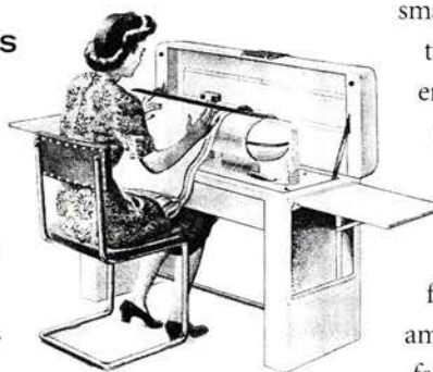
Roller ironers with one open end could iron clothes as well as flat work and were made by at least six manufacturers by the 1930s.
