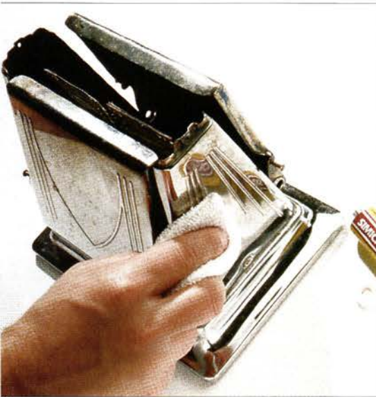
When toasters, stoves, and other cooking appliances overheat, the finish will often discolor with "heat bluing." Though this can be hard to remove, it may respond to polishes recommended for chrome. (Simichrome is one brand.)
