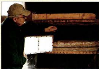
Inventor Doug Palmer holds a sample of Air Krete—dyed blue for quality control—showing how it will appear in the log walls.
