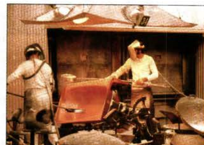
Kohler workers sift powdered enamel onto a super-heated cast-iron tub prior to refiring it.
