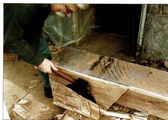
Switching to the broad axe, Doug hews away the kerfed oak to a square, smooth face. The offset handle of the axe allows him to work down the timber without hitting his knuckles.
