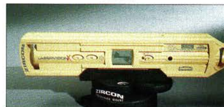
Top left: The Laser Jamb is a vertical rod that allows a rotary laser to trace a level line around a room. Top: Rotary lasers emit a single dot of light that, when rotated, reads as a continuous line. Above: Lasers mounted on a surveyor's tripod add high-tech to builders' and transit levels.
