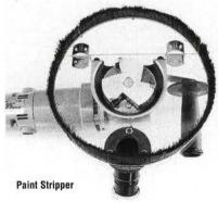
The Paint Stripper Accessory strips 1 sq. foot of paint in 15 seconds while collecting debris into a vacuum system.
