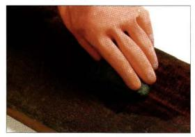
Fine steel wool (0000) is effective for cleaning finishes, but the steel "hairs" can catch between wood grains. Terry cloth and green 3M pads are other options.
