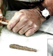
Above: Squeeze the copper around a bolt, screwdriver, or other object to obtain a halfround shape. A rattail file provides a handy form for a range of diameters, allowing you to exactly match your particular torus.
