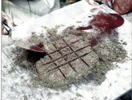
To measure pigments, divide the cake into smaller equal parts. As long as the sand is caked to a relatively even depth, you can segment it until you get to the desired ratio. For example, if your mortar-color testing samples call for a 1:32 ratio of pigment to sand, then divide the sand into 16 equal segments and scoop % of a %th segment out and fill the void with your pigment.
