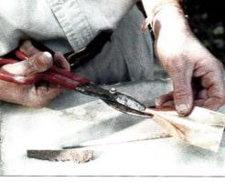
Left: Trim the tip with tin snips to reduce the surface area at the nose that forms the mortar. Above: Then trim back the adjacent metal. At this point, the strike tool begins to look like a paper airplane.
