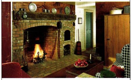
Tall and elegant... the fireplace that keeps you warm Based on the principles of Count Rumford, the streamlined throats and smoke chambers installed in masonry fireplaces built to our specifications radiate more heat to the room, waste less heat up the chimney and burn more cleanly.
