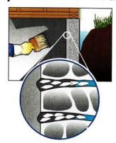
Concrete Waterproofing by Crystallization™
