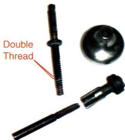
Though tricky to see, the groove on this J.L. Mott valve stem is actually a double thread. The mating tap is below.
