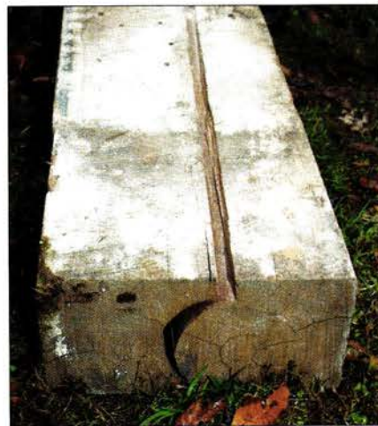
Old timbers can be both beautiful and rugged, but flaws such as this crack along a growth ring can eat into their value.
