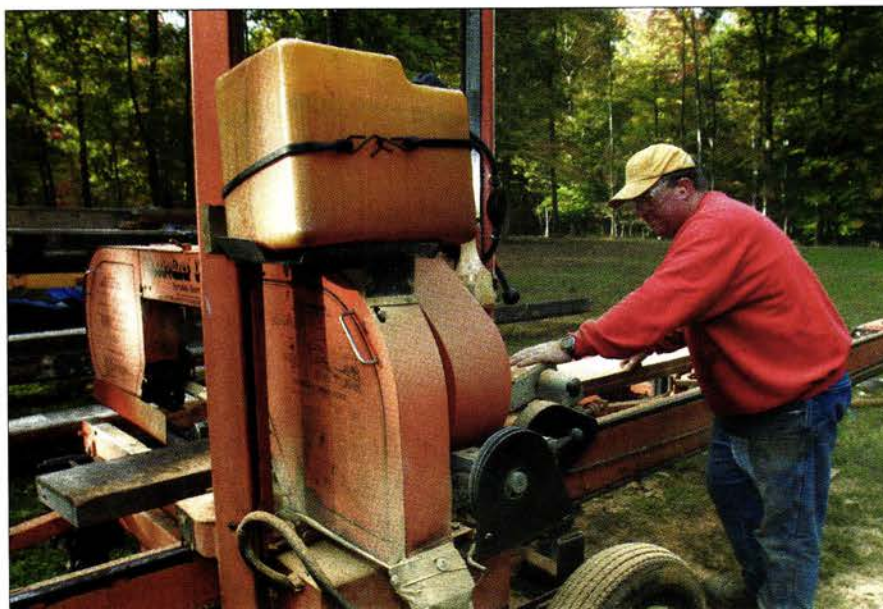
Mark saws 1 1/2' thick warehouse timbers to 1" thick planks. They'll later be planed to 3/16" to fill a customer's request for 1,500 square feet of flooring.
