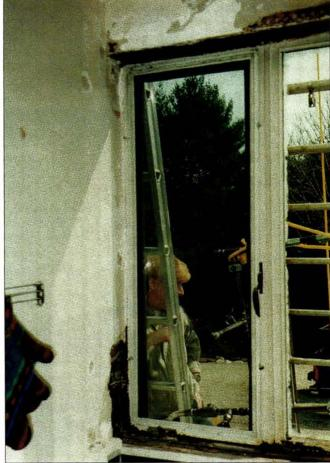
Our water test used a multiple nozzle spray rack hung from a ladder and calibrated to dispense a well-distributed film of water at a rate of 5 gallons per square feet per hour simulating heavy rain without the driving pressure of wind.
