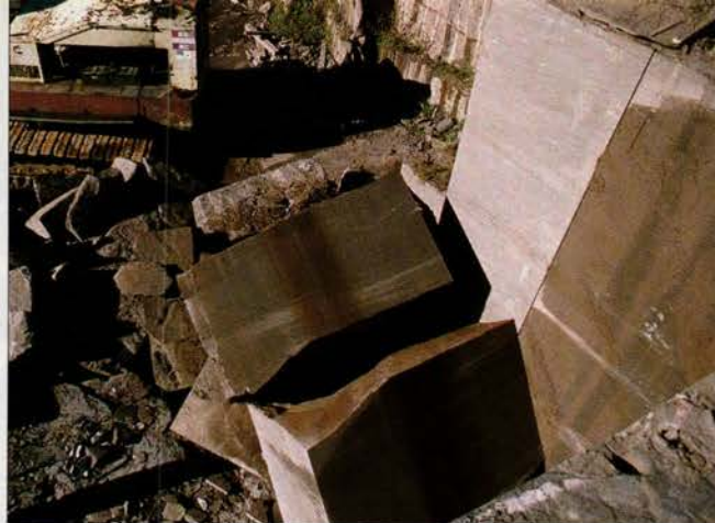
Enormous blocks are sawn out by a computer-aided machine and a diamond-studded wire that's threaded through 37'-long holes drilled vertically and horizontally into the cliff face.
