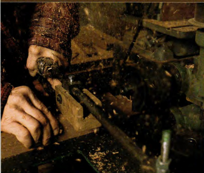
Above: Tenons are cut to fit into the square mortise. The tenoning machine cuts the top and bottom of each joint as the wood passes between the rotating cutters. Left: Oak Grove craftsman Will Arsnow demonstrates a tenoning machine that cuts the tenon on the sash rails.
