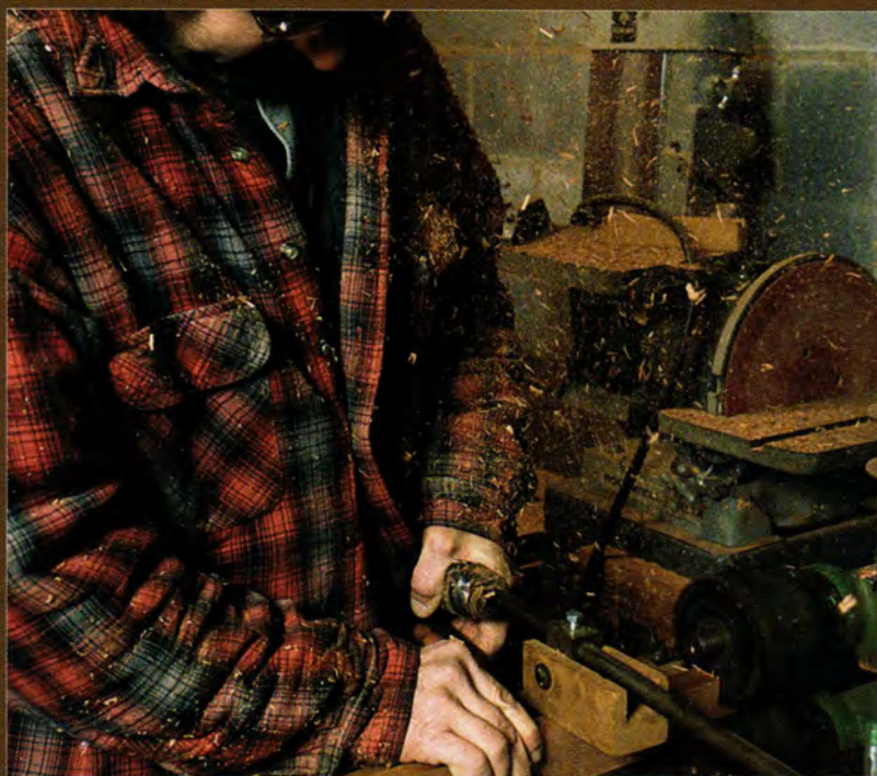
Above: Tenons are cut to fit into the square mortise. The tenoning machine cuts the top and bottom of each joint as the wood passes between the rotating cutters. Left: Oak Grove craftsman Will Arsnow demonstrates a tenoning machine that cuts the tenon on the sash rails.
