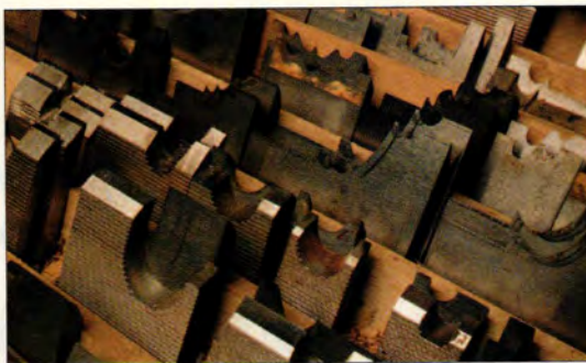
Custom-made cutters or tools are the hallmark of Oak Grove, each made to match original window molding profile.
