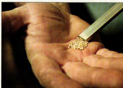
Hybrid spacers combine materials, such as this dessicant-filled aluminum, to improve efficiency.
