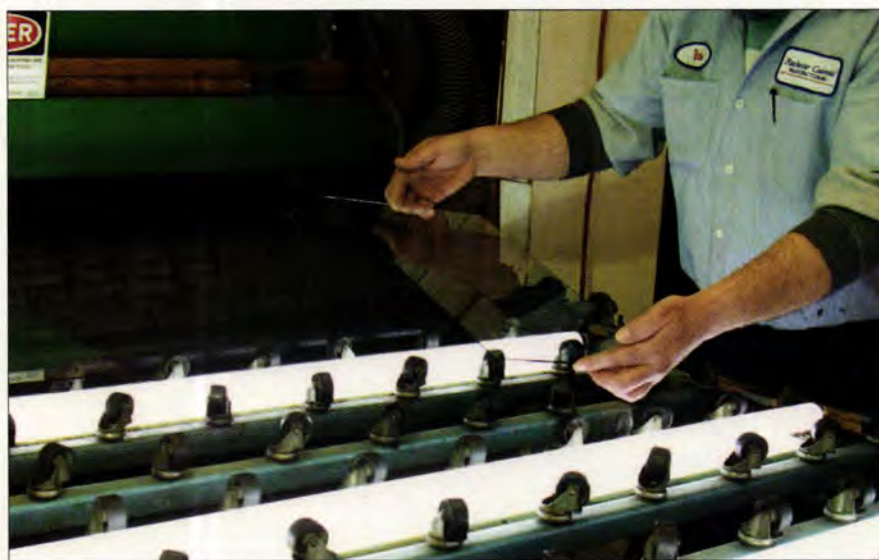
At Rochester Colonial, each piece of glass is meticulously machine washed, then inspected over special lights before it is assembled into an insulating window unit.
