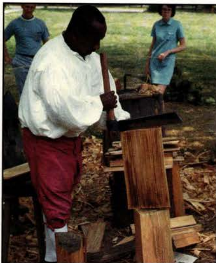
Working the wedge-like free down the timber bolt splits out a shingle.
