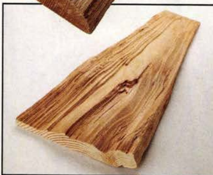
Clockwise from top left: The deeply corrugated face of a modern shake split with vertical grain (note butt end); a drawknife used to dress the face of a split shingle; machine-sawn shingle with characteristic circular blade marks; modern shake with random grain.
