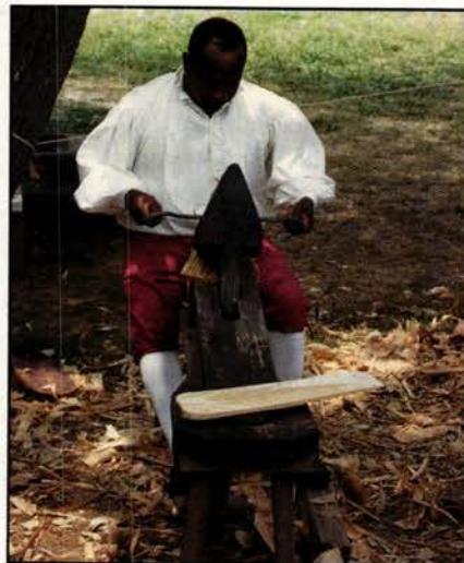
Clamped in a shaving horse, shingles are dressed smooth with a drawknife.
