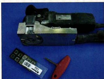
Paint shavers with narrow cutters and long soles allowed horizontal stripping on 4 1/2" shingles. Two tools with different cutter depths speeded work.
