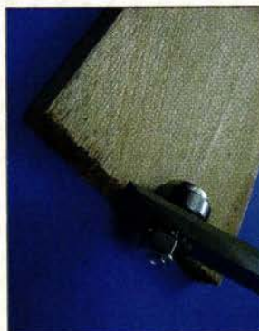
A sash chisel made for removing putty worked well for stripping butts.
