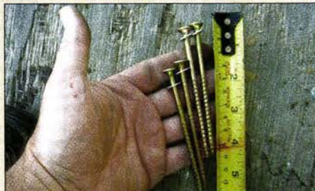
The sill Dutchmen needed to be anchored back to the framing; Spax screws had the required length and strength, as well as tips that start their own pilot holes.
