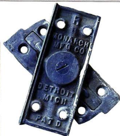
One of many versions from a 1916 patent, these Tabor sash centers set into the sash and window jamb. As seen in the Monarch model (above) the center screw adjusts the floating bar that holds the window at different angles.
