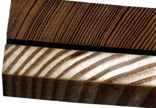
Concentrated rings (top) show how slowly old-growth lumber grew. Today's farmed trees (bottom) expand so quickly, natural preservatives have little time to accumulate.
