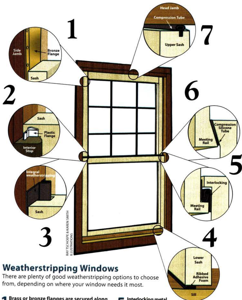
LEFT: Weatherstripping helps keep winter weather at bay on even the coldest days. ABOVE: The brass flange installed here is one of many ways to tighten up drafty areas around windows.
