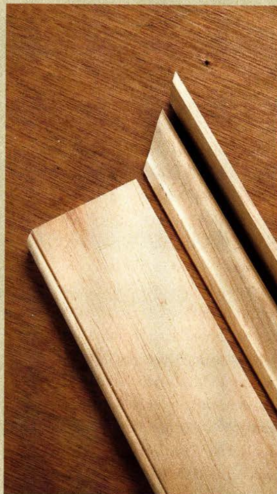
A look at the three separate elements shows how miter cuts on the lattice strip and the small profiled molding are aligned.
