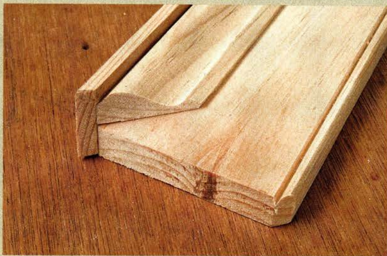
Stacked together, it's easy to see where the casing's corners meet and will be mitered together, including the small hip cut beneath the bead.
