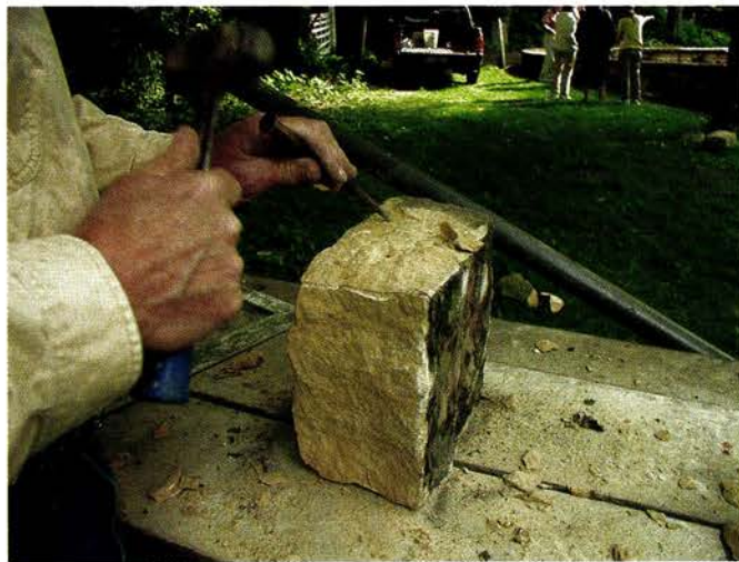
Clean up any high points along the sides of the new stone with a point chisel.
