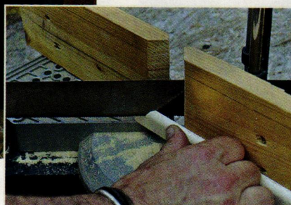
An old-fashioned miter box makes it easy to cut accurate angles in small pieces of trim like shoe molding returns.
