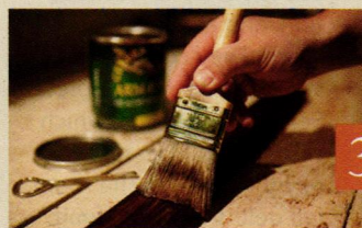
Brush on an oil-based urethane to prevent the dye from re-liquefying.
