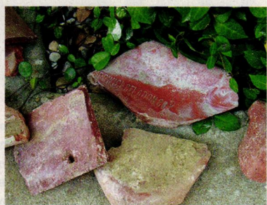
Tile fragments excavated in the garden confirmed the original roof's manufacturer—Ludowici—who was able to provide a perfect match.
