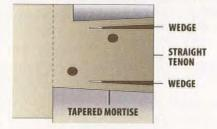
This wedged through-tenon drawbored joint has the wedges driven into kerfs in the tenon, spreading the tenon into a dovetail shape to fill the tapered mortise. This is a solid joint that almost always requires removing the wedges before disassembly, even if the joint is loose.
