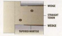
This wedged through-tenon drawbored joint has a straight tenon and a tapered mortise. Wedges are used to tighten the tenon in the mortise.
