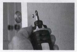
Dialing the clutch ring to a higher number cranks up the torque output. The maximum setting (drill mode) bypasses the clutch and is usually marked with a drill bit icon.
