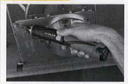
The pistol grip should be the default, but switch to the inline form for maximum reach in tight spaces. Adjust the clutch down or hold on tight: In drill mode or at high clutch settings, the tool can be easily wrested from your grip when the fastener seats.
