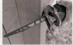
To get control of the saw's reciprocating motion, get a tight grip and firmly press the shoe into the work for the duration of the cut. The piece being cut—whether flimsy metal or a beefy fence post—acts as a sort of fulcrum that enables cutting.
