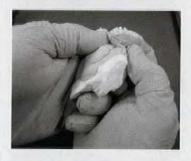
For the best performance, resinto-hardener proportions need to be accurate and mixed thoroughly. Take equal amounts of part A and part B from each container, and knead this ball until the color is even throughout. After you start kneading, don't reach back into either container without putting on fresh gloves.
