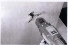
To get the most drilling and driving out of your tool, use its controls to your maximum advantage. High and low gear determine the torque vs. speed output, and the clutch settings let you dial in the depth-ofdrive force to seat fasteners just right.
