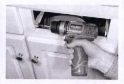
For boring holes or driving fasteners in all sorts of tight spots, a subcompact drill/driver is an ideal tool. Using 1-inch bits (if the tool fits them) is an easy way to get additional room.
