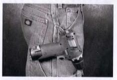
These tools don't come with a lot of extras, but one feature that comes in handy is a belt hook that can be attached to either side of the handle. Besides making it easier to climb a ladder with the tool, it also keeps the tool right at hand.
