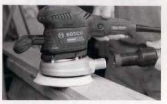
Most of these sanders are designed to collect dust two ways: via a built-in canister or by connecting them to a shop vac. Switching to a vacuum connection is as simple as removing the canister and replacing it with the vacuum hose.
