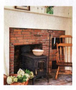
Even a small fireplace can take a freestanding **stove**, set slightly forward of the firebox. Most are B-vented through the flue; some modern ones direct vent.
