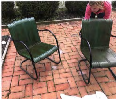
2. Hand-sanding with 0 and 00 grades of steel wool removed a surprising amount of rust, revealing the underlying paint colors.
