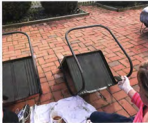
3. Here the homeowner and her friend apply the first coat of Penetrol, a paint additive that adds a soft, sealed finish to metal.
