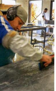
TOP [left] Leonardo Ribeiro, production manager and shop foreman, lowers a stone slab into position on the cutting bed. (right) A monitor shows both worker and CNC machine exactly where cuts are to be made on the slab. ABOVE The sharp edges of a grooved countertop are hand-sanded by Angel Paguay. INSET A native of Brazil, Roger Teixeira has been in the soapstone business for 25 years.
