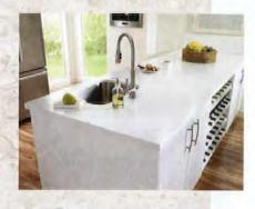
WilsonArt's Angel Falls solid surfacing material (background) resembles marble. RIGHT Corian can be thermoformed, which means it's easy to create integral sinks, grooves, and changes in surface height.
