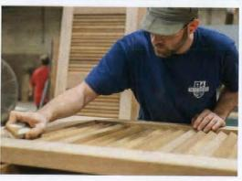
FAR LEFT After the stiles, rails, and louvers are trimmed to size, individual components in the Shutters-in-a-Box system from Aeratis assemble onsite in as little as 30 minutes per shutter. LEFT A worker at Withers Industries sands a pair of custom wood shutters. TOP Deeply beveled panels, rabbeted channels, and properly placed, functional hardware are all hallmarks of period-specific shutters, like these from Timberlane.
