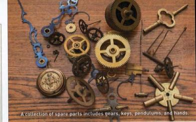
eight-day clock should be wound once a week, as the mainspring loses power after seven days. A 30-hour clock should be wound daily; a good routine is to wind it every night before bedtime. The key should fit tightly. If it is loose, slipping can occur during winding and the ratchets will not seat properly, potentially causing a sudden unwinding of the mainsprings.
