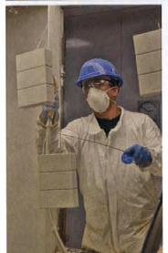
ABOVE At Runtal North America's factory, Duane Barnard TIG-welds fins to the front panels. LEFT Completed panels and trim covers pass through the enclosed paint station, where they're manipulated by Miguel Dia and sprayed in a single pass. Panels dry briefly, then the color is baked on at 400 degrees.
