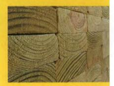
**ABOVE** A standard building material, PT lumber can be used in contact with the ground and is affordably priced.
