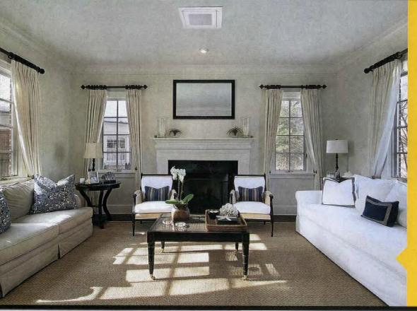
With minimal ducting, a mini-split compact cassette evenly distributes cool or warm air through a vent not much larger than a conventional forced air return.
