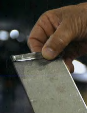
A worker holds two wedge-shaped nails at opposite ends, demonstrating how the nails are cut to make the most efficient use of steel strips.
