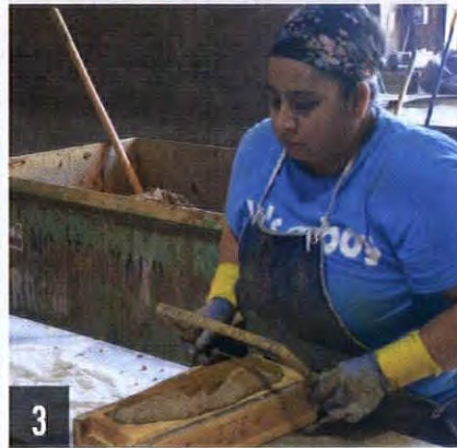
ABOVE (steps one through three) Nancy Hernandez raises a wedge-shaped slug of clay, throws it into a wooden brick mould, then cuts off the excess with a wire cutter. LEFT Carmen Alba makes an Old Carolina Thin Brick by slicing the edge off a solid, hand-made brick.
