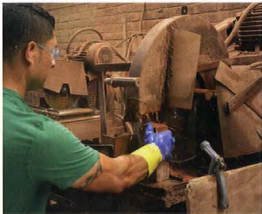
ABOVE (steps one through three) Nancy Hernandez raises a wedge-shaped slug of clay, throws it into a wooden brick mould, then cuts off the excess with a wire cutter. LEFT Carmen Alba makes an Old Carolina Thin Brick by slicing the edge off a solid, hand-made brick.
