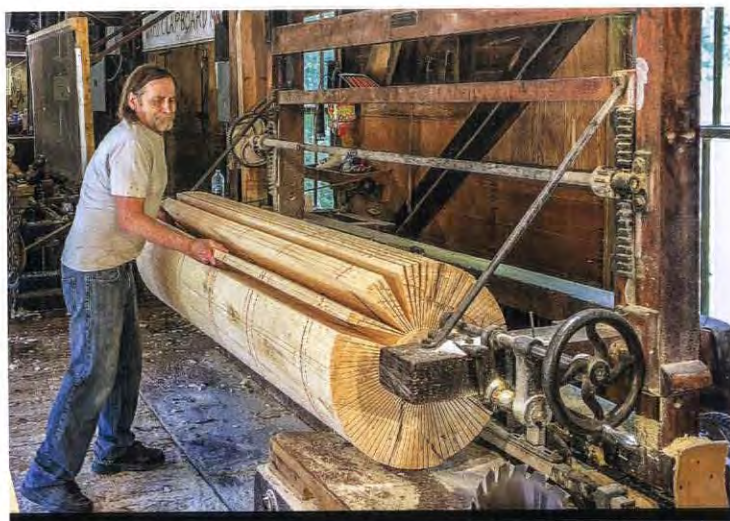
LEFT Long-time sawyer Bob Pierce operates the radial saw at Ward Clapboard Mill in Moretown, Vermont. Good-looking and stable, clapboards cut this way actually last.
